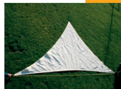
Then the side length is tensioned and measured under tension. The measuring tape is positioned at the outermost point of the sail corner- i.e. incl. belt strap loop, D-ring or carbine.
